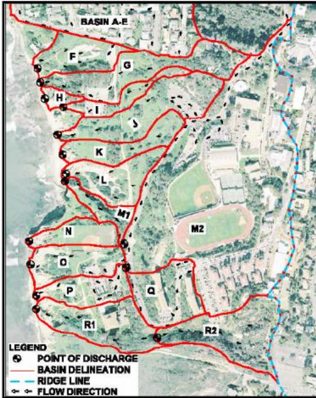
Figure 1. Hillside Park drainage basins presented in the Dudek & Associates Hydrology Study, based on a 1999 topographic map. The drainage basins for the Linear Park are shown on Dudek schematic concept diagrams showing drainage system alternatives. Drainage basin boundary lines in some cases do not appear to represent actual boundaries to flow, but may have been used for engineering flow calculations.
