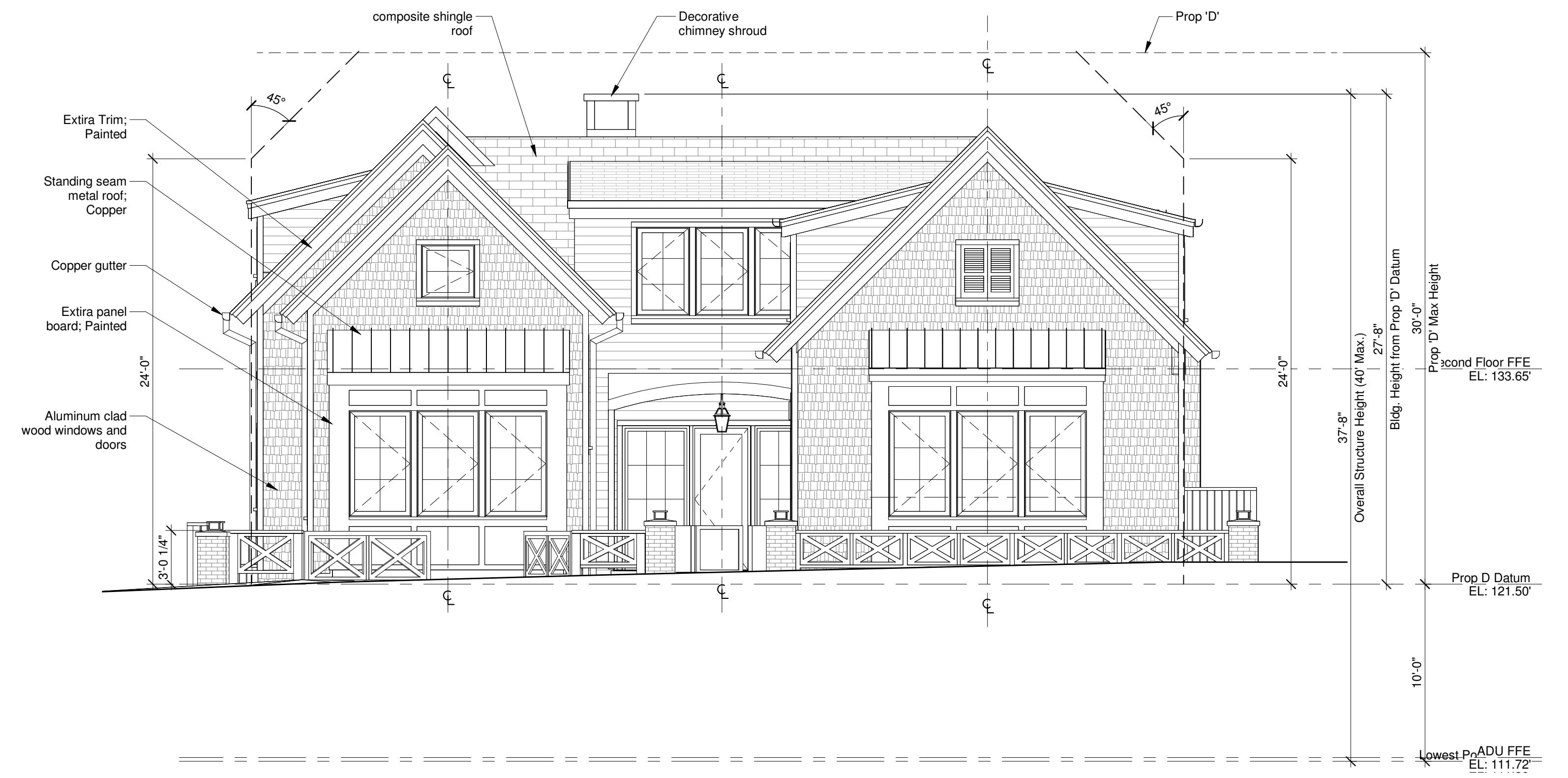
1 East Elevation (Front) 3/16" = 1'-0"
